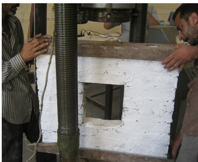
Figure (15) A steel beam as C-channel for transfer the uniform load to wall.
