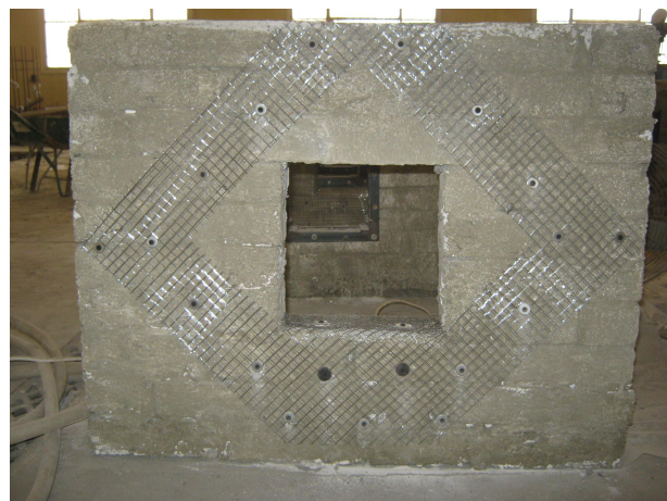
Figure (8) Details of the used rehabilitation technique using (2, 3, 4) layers of steel wire mesh as diagonal shape fixed with fisher bolts.
