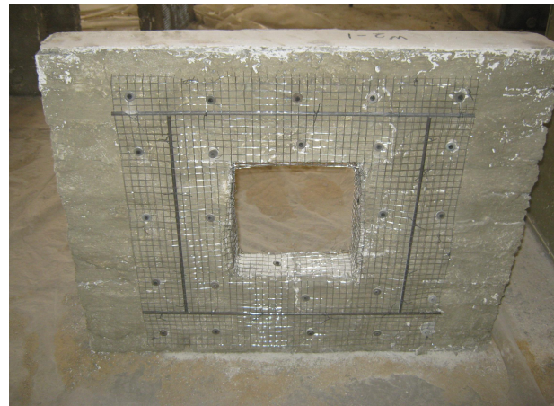
Figure (9) Details of the used rehabilitation technique using two layers of steel wire mesh with 106 additional external steel bar in between.
