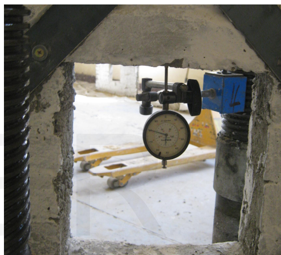
Figure (13) The used dial gauge for measuring lintel deflection.
